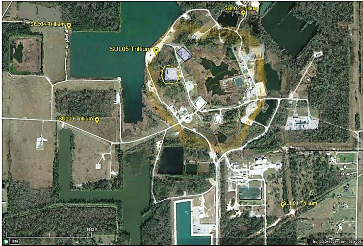
Figure 1. Google map image showing the location of the broadband seismic (Trillium Compact Sensors, yellow symbols and labels) stations near and at the Sulphur Mines Salt Dome.
