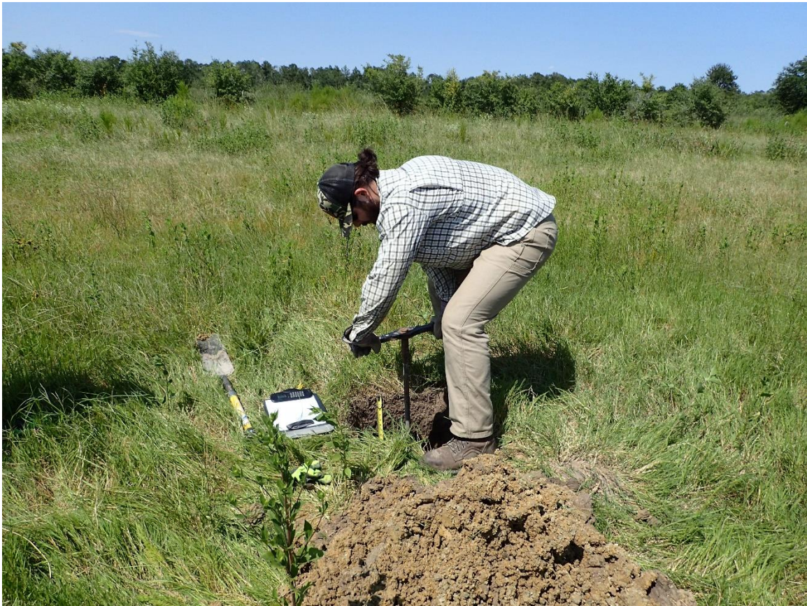
Photo B-39. Hand auger at H-05.
