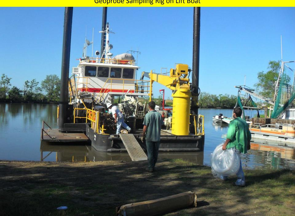
Geoprobe Sampling Rig on Lift Boat
