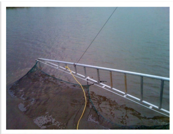
IMG_0487: Submerged net on extended boom being pulled through water at location TR-05
