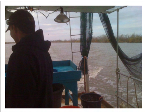
IMG_0495: Detail of sorting table, fish collection basket, and nets on trawling boat
