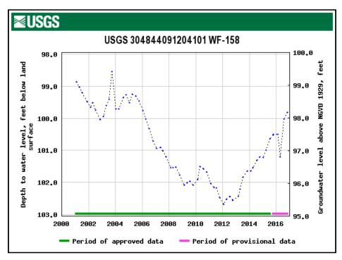
Fig. 13.4: Monitor well in the 1700-foot sand, Evangeline Equivalent Aquifer System, West Feliciana Parish, showing slight downward trend since 2001 and upward trend since 2012. Source: USGS.
