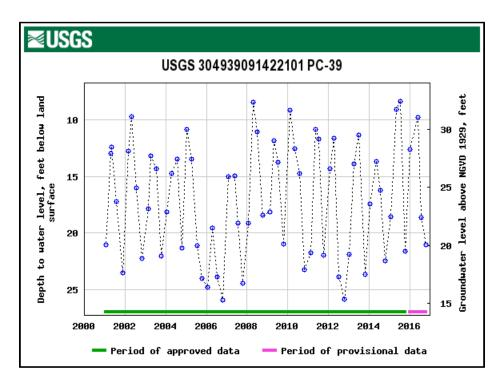
Fig. 12.5: Monitor well in the 2000-foot sand, Jasper Equivalent Aquifer System, Pointe Coupee Parish, showing downward trend since 2001 but upward movement since 2013. Source: USGS.
