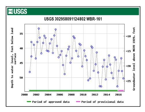
Fig. 11.5: Monitor well in the 1200-foot sand, Evangeline Equivalent Aquifer System, West Baton Rouge Parish, showing downward trend since early 2000s. <u>The Evangeline Equivalent is the most heavily used</u> groundwater resource in West Baton Rouge. Source: USGS.
