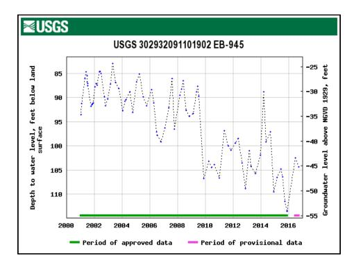
Fig. 10.5: Monitor well in the 800-foot sand, Evangeline Equivalent Aquifer System, East Baton Rouge Parish, showing relative stasis since 2010. Source: USGS.
