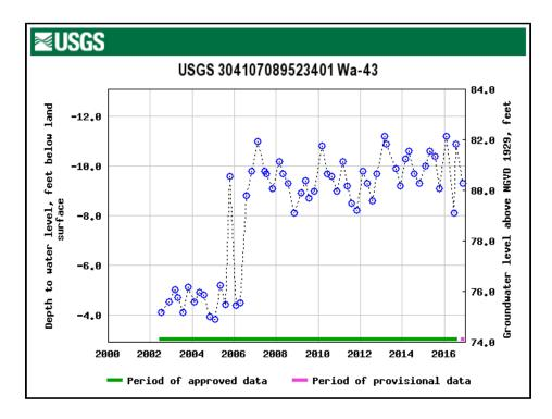
Fig. 18.5: Monitor well in the Amite Aquifer, Jasper Equivalent Aquifer System, Washington Parish, showing water level trending upward since 2001. Source: USGS.
