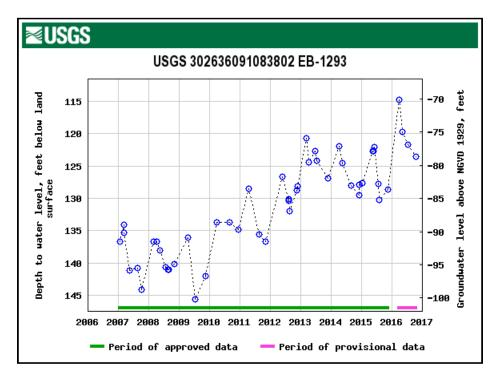
Fig. 10.7: Monitor well in the 1700-foot sand, Evangeline Equivalent Aquifer System, East Baton Rouge Parish, showing slight upward trend over the past two years. Source: USGS.
