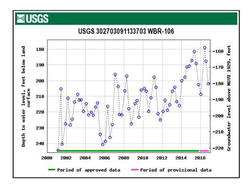
Fig. 11.9: Monitor well in the 2000-foot sand, Jasper Equivalent Aquifer System, West Baton Rouge Parish, showing downward trend since early 2000s but relative stasis since 2012. Source: USGS.
