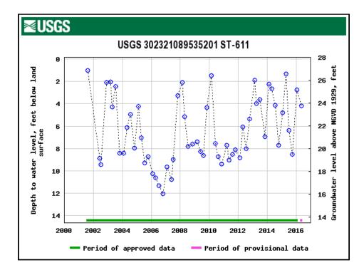
Fig. 19.4: Monitor well in the Upland Terrace Aquifer, Chicot Equivalent Aquifer System, St. Tammany Parish, showing relative stasis in water levels over last decade. Source: USGS.
