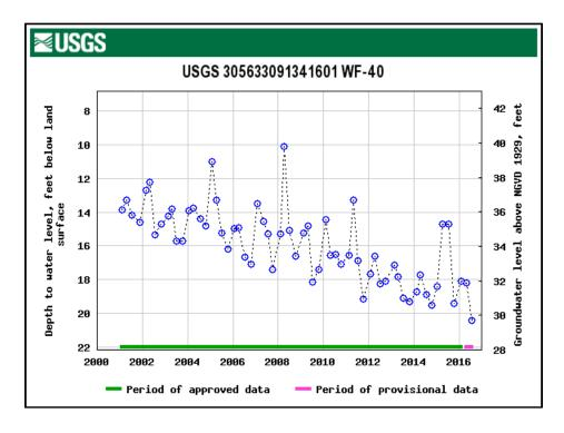
Fig. 13.6: Monitor well in the 2400-foot sand, Jasper Equivalent Aquifer System, West Feliciana Parish, showing relative stasis through first decade of 2000s, followed by drawdown since 2014. Source: USGS.
