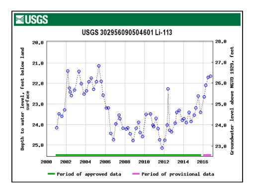
Fig. 15.6: Monitor well in the 1700-foot sand, Evangeline Equivalent Aquifer System, Livingston Parish, showing water level decline and recovery, and decline again, over the past decade. Source: USGS.
