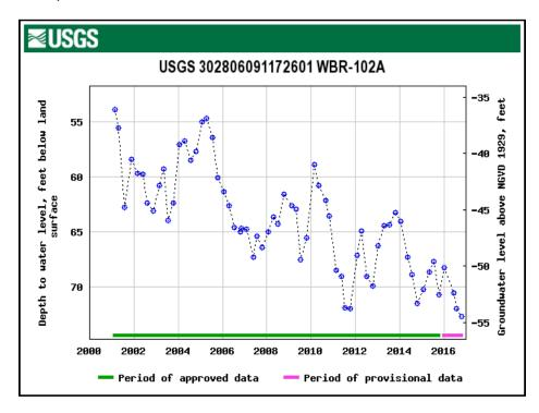
Fig. 11.7: Monitor well in the 1700-foot sand, Evangeline Equivalent Aquifer System, West Baton Rouge Parish, showing steep downward trend since 2012. Source: USGS.
