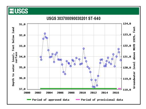
Fig. 19.5: Monitor well in the Big Branch Aquifer, Evangeline Equivalent Aquifer System, St. Tammany Parish, showing relative stasis in water level since 2001. Source: USGS.
