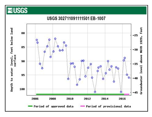
Fig. 10.6: Monitor well in the 1500-foot sand, Evangeline Equivalent Aquifer System, East Baton Rouge Parish, showing upward trend since 2007. Source: USGS.
