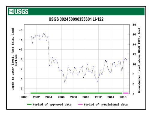
Fig. 15.4: Monitor well in the 400-foot sand, Chicot Equivalent Aquifer System, Livingston Parish, showing water level decline and recovery over the past decade. Source: USGS.
