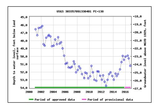
Fig. 12.6: Monitor well in the 2800-foot sand, Jasper Equivalent Aquifer System, Pointe Coupee Parish, showing downward trend since 2001. Source: USGS.
