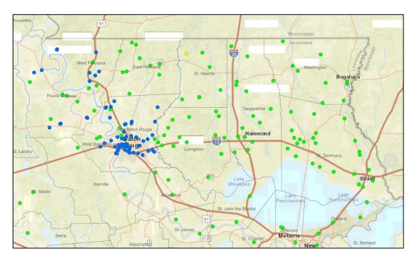
Fig. 6: The groundwater monitor network in the 10-parish area overlying the Southern Hills Aquifer System. Green dots indicate wells monitored by the USGS for DOTD (including wells added through the DNR/USGS expanded monitoring project). Blue dots represent wells monitored by the USGS for the Capital Area Ground Water Conservation Commission. Source: USGS.
