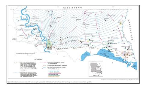
Fig. 7: Groundwater flow in the 1500- and 1700-foot sands of the Southern Hills Aquifer System (Evangeline Equivalent). L.B. Prakken, Louisiana ground-water map no. 17: Generalized potentiometric surface of Kentwood the aquifer system and the "1500-foot" and "1700-foot" sands of the Baton Rouge area in southeastern La., March-April 2003, 2004.
