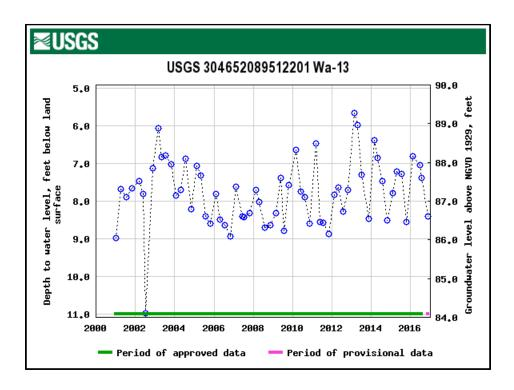
Fig. 18.4: Monitor well in the Lower Ponchatoula, Evangeline Equivalent Aquifer System, Washington Parish, showing water level rise and relative stasis over last decade. Source: USGS.
