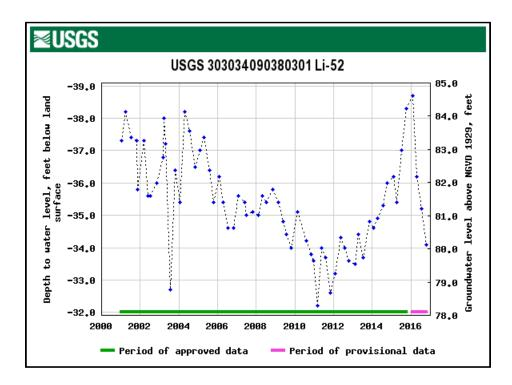
Fig. 15.7: Monitor well in the 2400-foot sand, Jasper Equivalent Aquifer System, Livingston Parish, showing relative stasis in water levels since 2001. Source: USGS.
