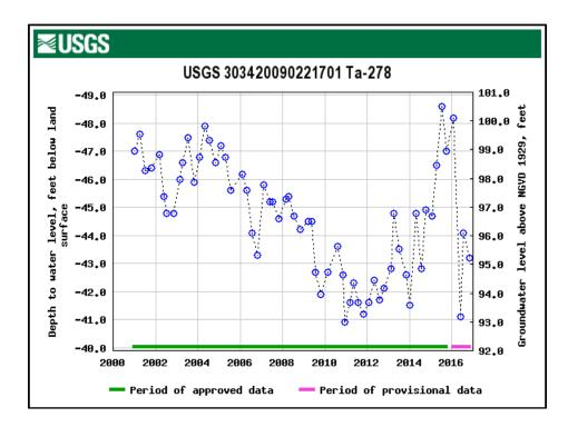
Fig. 17.5: Monitor well in the Covington Aquifer, Evangeline Equivalent Aquifer System, Tangipahoa Parish, showing water level drawdown and relative stasis since 2002. Source: USGS.
