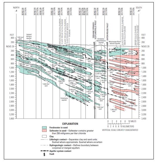
Fig. 2: Generalized north-to-south hydrogeologic section through the western part of the Southern Hills Aquifer System, showing the Chicot, Evangeline, and Jasper Equivalent System classifications and the generalized extent of saltwater in local sands. Source: White, *Southern Hills Regional Aquifer System*.
