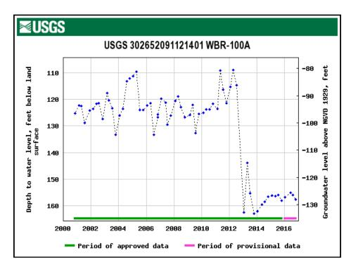
Fig. 11.8: Monitor well in the 2000-foot sand, Jasper Equivalent Aquifer System, West Baton Rouge Parish, showing upward trend since early 2000s. Source: USGS.
