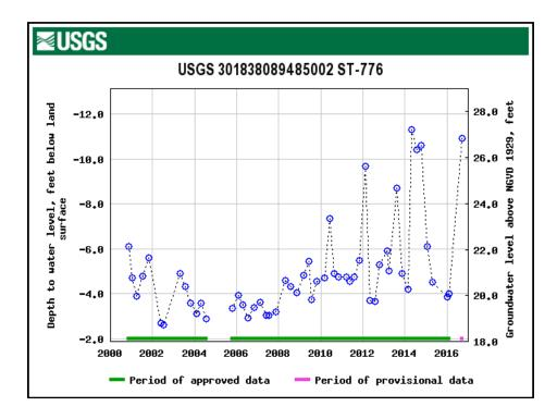
Fig. 19.8: Monitor well in the Tchefuncte Aquifer, Jasper Equivalent Aquifer System, St. Tammany Parish, showing water level rise and downward trend since 2011. Source: USGS.
