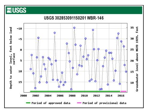
Fig. 11.4: Monitor well in the 600-foot sand, Chicot Equivalent Aquifer System, West Baton Rouge Parish, showing downward trend since early 2000s. Source: USGS.
