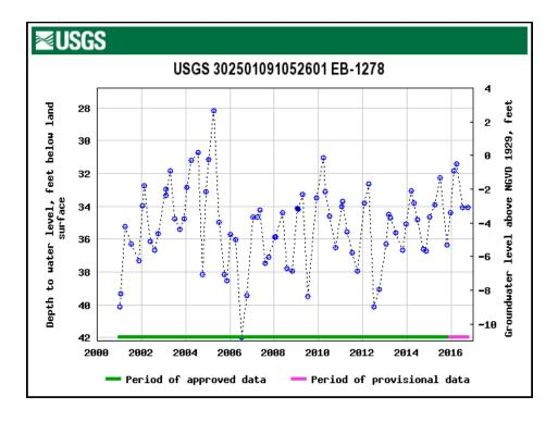
Fig. 10.4: Monitor well in the 600-foot sand, Chicot Equivalent Aquifer System, East Baton Rouge Parish, showing expected declines since 2000, and relative stasis since 2010. Source: USGS.
