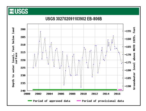
Fig. 10.9: Monitor well in the 2800-foot sand, Jasper Equivalent Aquifer System, East Baton Rouge Parish, showing decline, relative stasis, and upward trend since 2012. Source: USGS.
