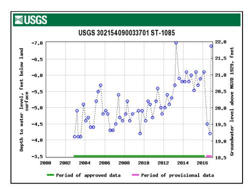
Fig. 19.7: Monitor well in the Lower Ponchatoula Aquifer, Evangeline Equivalent Aquifer System, St. Tammany Parish, showing upward trending water level since 2008. Source: USGS.
