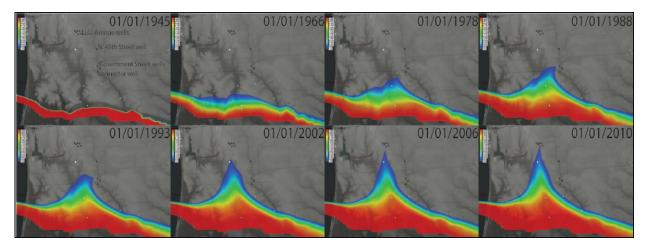
Fig. 9, Saltwater intrusion approach towards Lula Pumping Station in the 1500-foot sand, Baton Rouge, 1945-2010. Dark blue represents a concentration of 250 mg/l, the upper limit of EPA's safe drinking water guideline. Source: Frank T.-C. Tsai, et al., "Feasibility Study of Scavenging Approach to Stop Saltwater Toward Water Wells," 2012.
