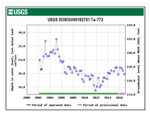
Fig. 17.6: Monitor well in the Amite Aquifer, Jasper Equivalent Aquifer System, Tangipahoa Parish, showing water level drawdown, rise, and relative stasis since 2012. Source: USGS.
