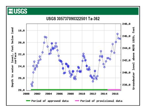
Fig. 17.4: Monitor well in the Covington Aquifer, Evangeline Equivalent Aquifer System, Tangipahoa Parish, showing water level drawdown and rise since 2001. Source: USGS.
