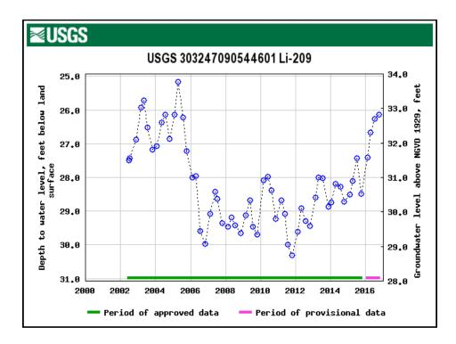
Fig. 15.5: Monitor well in the 1200-foot sand, Evangeline Equivalent Aquifer System, Livingston Parish, showing water level decline and recovery over the past decade. Source: USGS.
