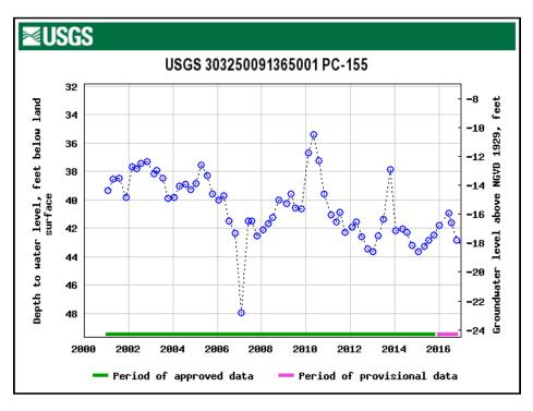
Fig. 12.4: Monitor well in the 1500-foot sand, Evangeline Equivalent Aquifer System, Pointe Coupee Parish, showing relative stability since 2001. Source: USGS.
