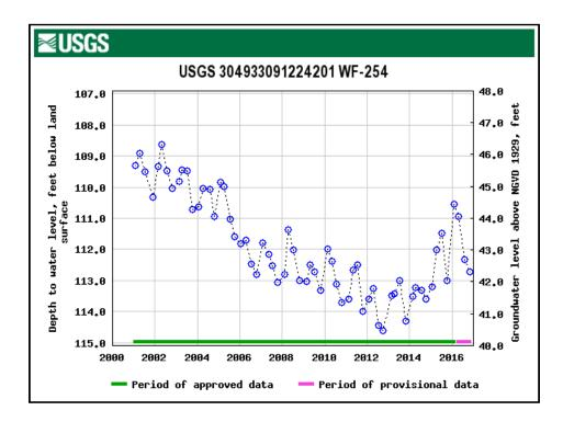
Fig. 13.5: Monitor well in the 2000-foot sand, Jasper Equivalent Aquifer System, West Feliciana Parish, showing slight downward trend since 2001. Source: USGS.
