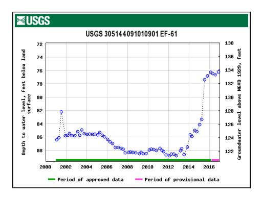
Fig. 14.4: Monitor well in the 2800-foot sand, Jasper Equivalent Aquifer System, East Feliciana Parish, showing relative stasis over the past decade. Source: USGS.
