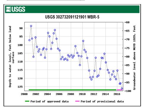
Fig. 11.6: Monitor well in the 1200-foot sand, Evangeline Equivalent Aquifer System, West Baton Rouge Parish, showing downward trend since early 2000s. Source: USGS.
