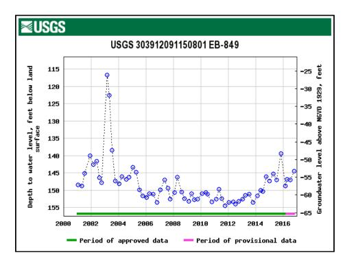
Fig. 10.8: Monitor well in the 2400-foot sand, Jasper Equivalent Aquifer System, East Baton Rouge Parish, showing relative stasis since 2000. Source: USGS.
