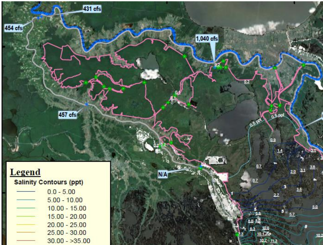
Figure 6-22. Portion of LPBF Hydrocoast Map providing a summary of water quality results obtained at a number of points around Lake Pontchartrain during the week starting May 23, 2016. The light blue line south of Lake Salvador is the 0.5 ppt isohaline showing that the LDA EMU as well as Lake Salvador were freshwater at this time. Weekly Hydrocoast Maps for the Barataria Basin can be downloaded at file:///C:/Users/gpkemp/Documents/EstCoastShelfSci/Revisions/HcBb29May2016psu.pdf.
