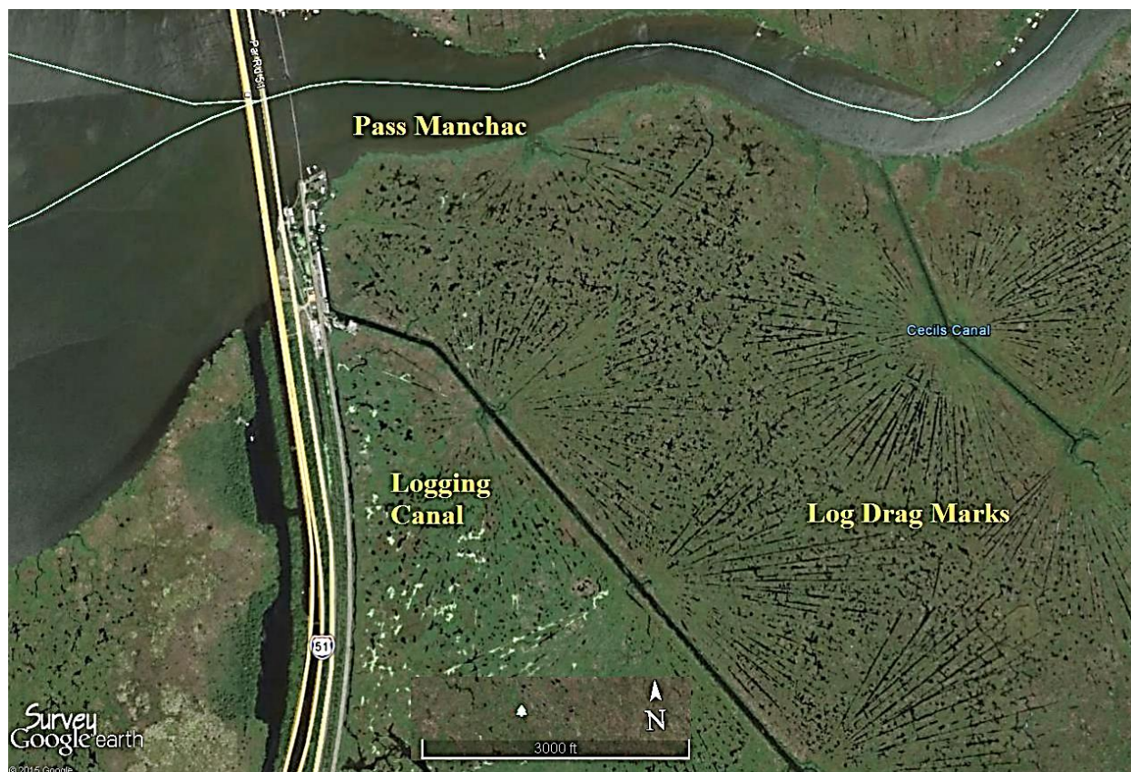
Figure 6-12. Logging canals and drag marks in the MS EMU south remain visible in marsh south of Pass Manchac 100 years after they were created. The swamp never regrew in this area. The railroad and Hwy. 51 are built on earthen causeways that parallel the I-55 elevated highway visible to the left near the east shore of Lake Maurepas.
