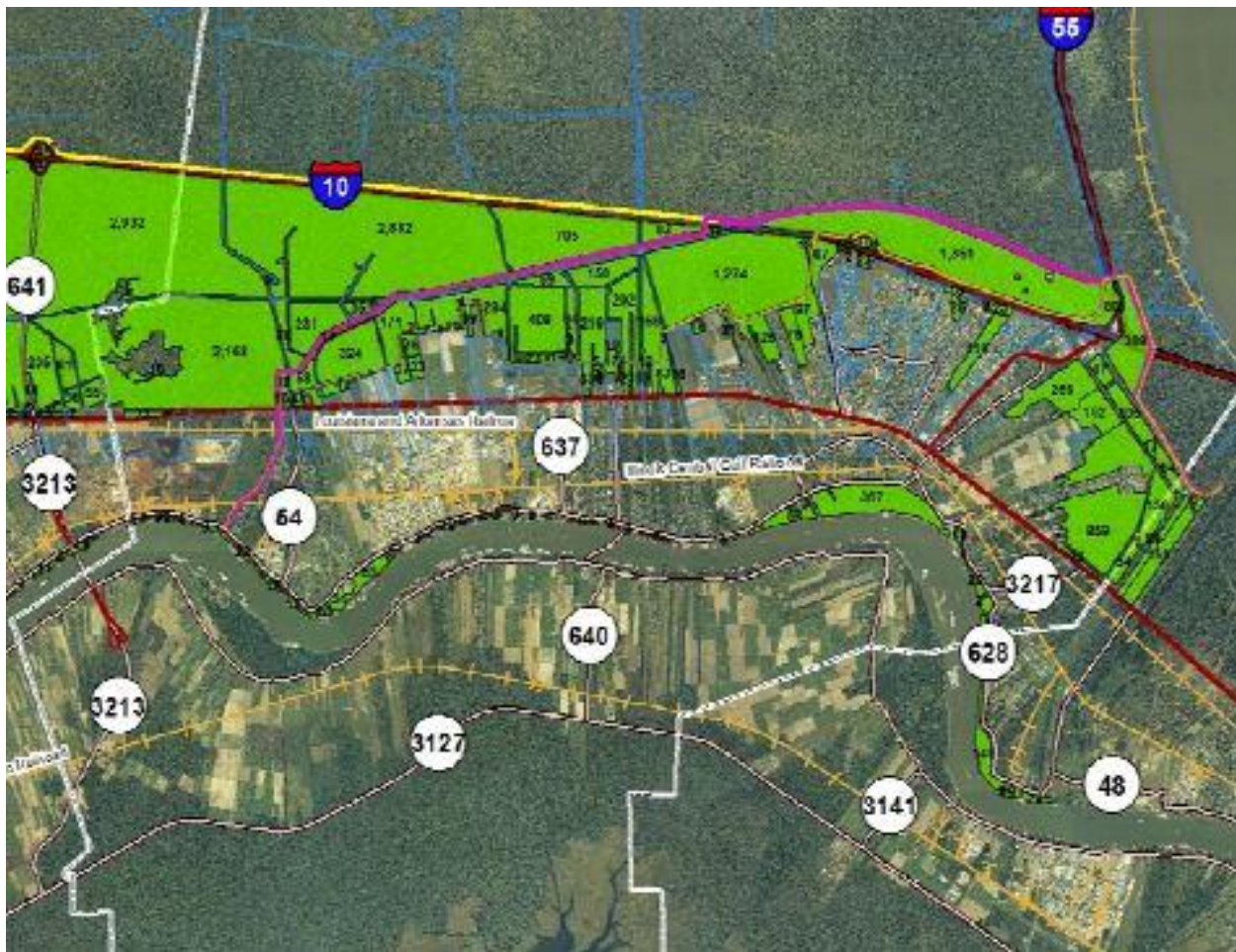
Figure 4-4. Wetlands (green) affected by the USACE West Shore Lake Pontchartrain Hurricane Risk Reduction Plan levee (shown in purple). Image Source: USACE
