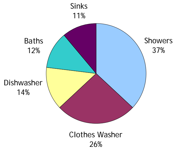
Figure 9-1 Typical Breakdown of Hot Water Use
