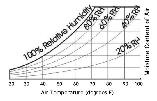
Figure 2-8 Winter Dew Point Temperature Inside Walls 100% Relotive Humid Moisture Content of Air 00 20%8 3 20 30 50 70 40 60 80 90 100 Air Temperature (degrees F)
