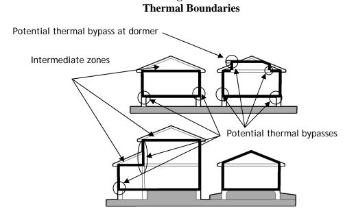
The designer and builder must direct the subcontractors about how to install continuous air and ductwork sealing materials, insulation, moisture retarders, drainage systems, and other building materials. The air quality and durability of a home depend vitally on how well these boundaries are installed and maintained.
