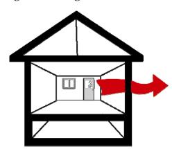
Figure 2-1 Home Losing Heat through Conduction in Winter
