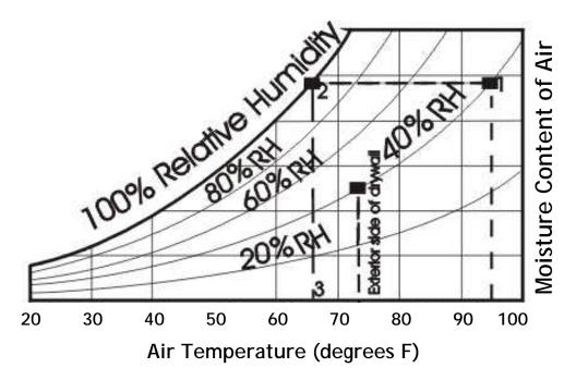
Figure 2-9 depicts a similar case in summer. If the interior air is 75°F, and outside air at 95°F and 40% relative humidity enters the wall cavity, will condensation occur on the exterior side of the drywall, which would be about 73°F? Using the psychometric chart, we find that the dew point of the outside air leaking into the wall cavity would be about 67°F. Since the drywall temperature is greater than the dew point, condensation should not form.
