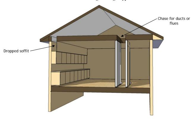
Figures 4-8, 4-9, and 4-10 show key areas that must be sealed to create an effective air barrier. The builder must clearly inform his or her subcontractors and workers of these details to ensure that the task is accomplished successfully. Make certain all sealants have at least 40-year service lives.
