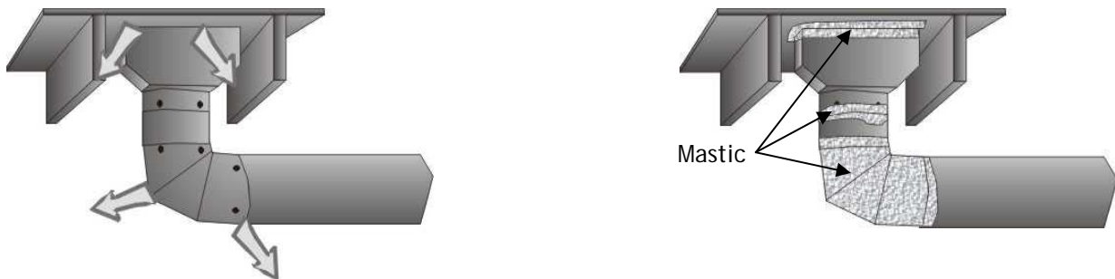
Figure 8-10 Sealing Leaky Boots
