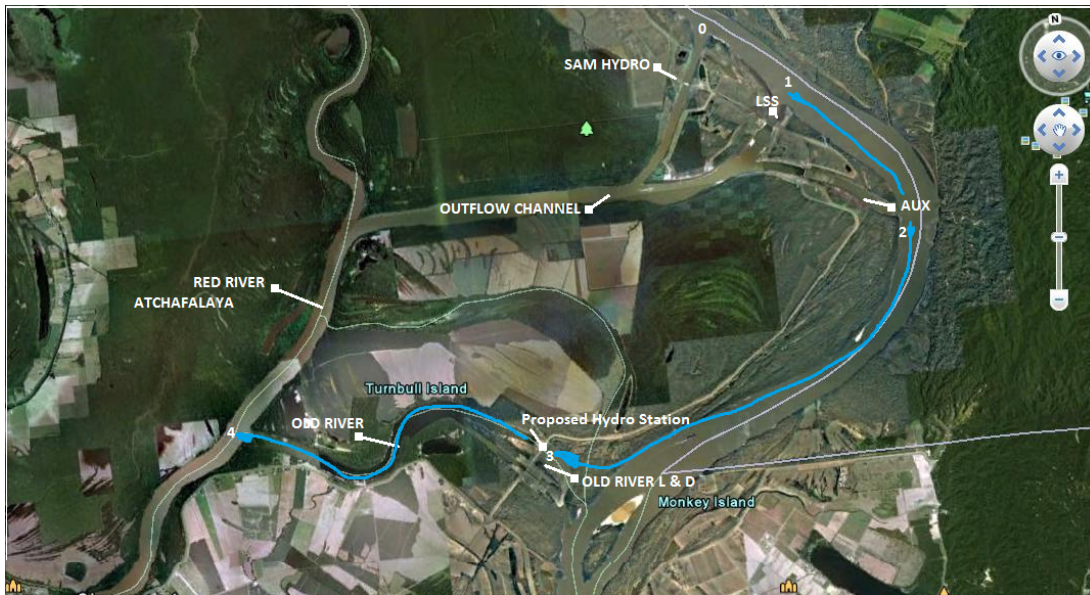
Mississippi River in the Old River Control Complex area with various existing flow diversion structures: (0) The Sidney A. Murray Hydroelectric Station, (1) The Low Sill Structure, (2) The Auxiliary Structure and (3) The Proposed Hydro Station at The Navigation Lock and Dam connecting Old River to the Red - Atchafalaya River.
