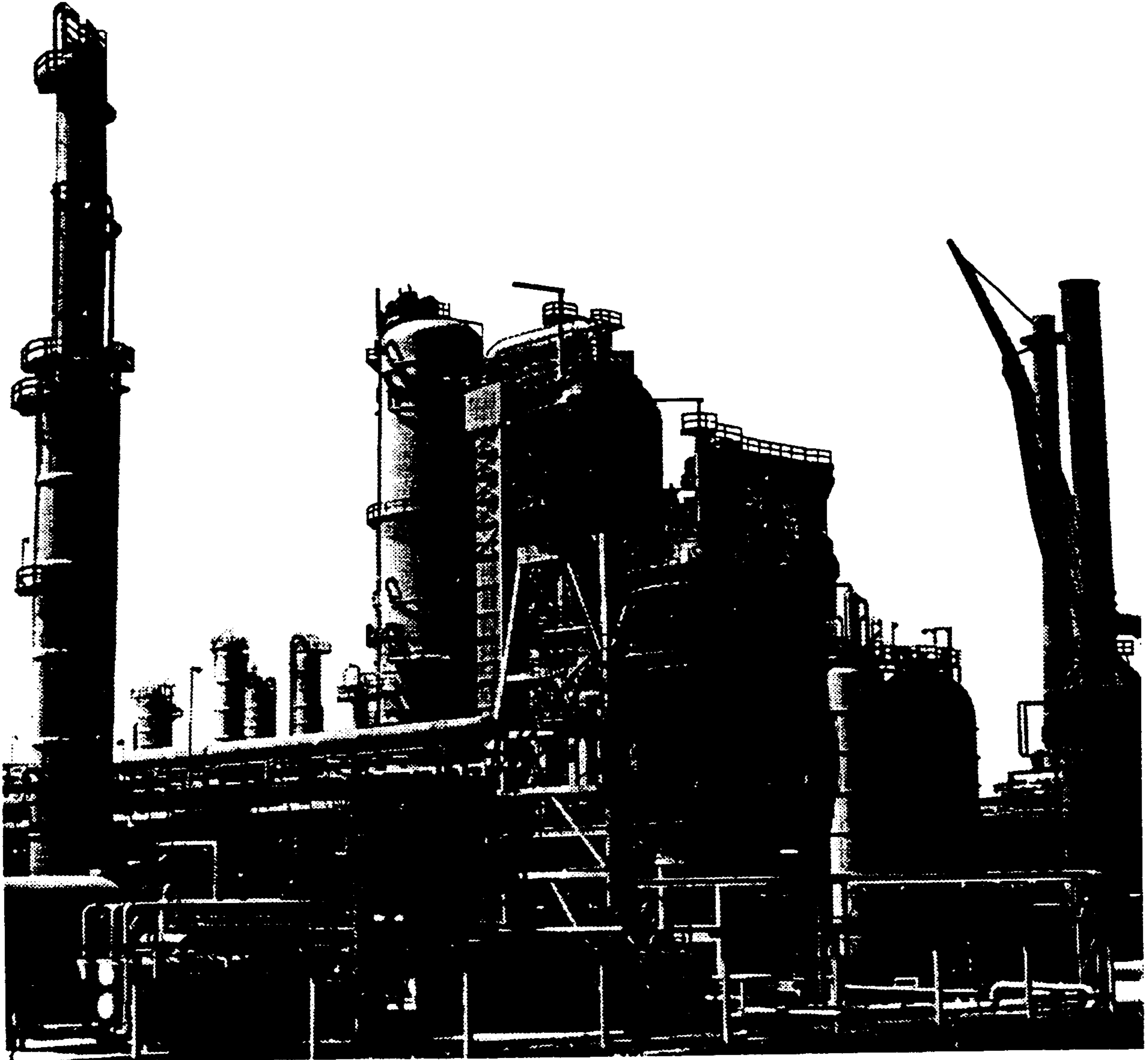
A catalytic cracking unit, used to increase the yield of gasoline from crude oil.
