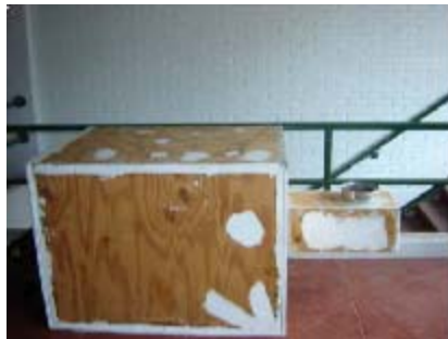
Figure 10-1. Leak Test Chamber 1
