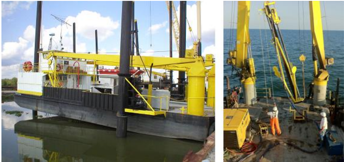
Figure 3 - Photographs of EBI® liftboat. Right photo shows OSI crew recovering a core utilizing one of the stern-mounted cranes permanently installed on the vessel.
