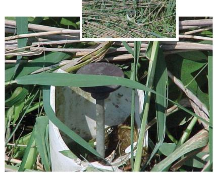
Position determined by using Real-time Kinematic (RTK) survey from Temporary Flypoint "BILL"
